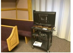
2. Mount the camera as shown. Be careful not to damage the monitor screen. Turn the cart and aim the camera towards the pulpit.
